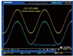
PCS-1000I vs. Current Probe for Measurement
