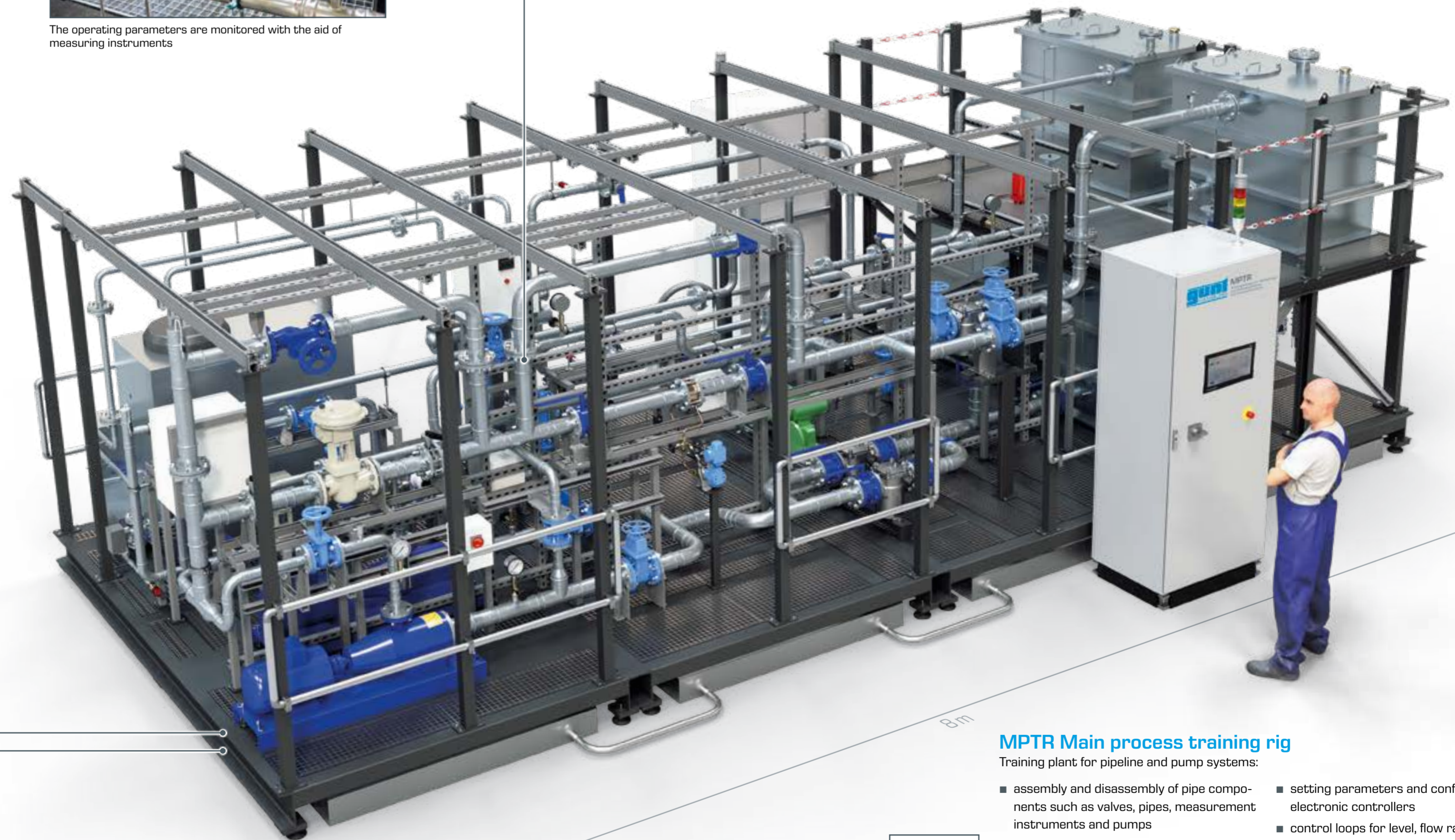
With different fittings different operating conditions can be set
