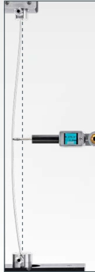
Euler case 3: bar fixed at the top, pinned at the bottom; the buckling of the test bar is measured
