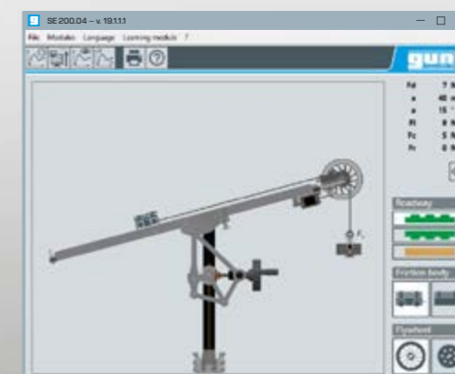
GUNT software: forces and inclination angles, selection of the friction surface and flywheels
